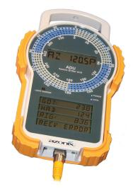
**The Azonix Drilling Unit (ADU)** was developed as a cost effective directional drilling display to help the driller validate the azimuth and inclination. Sporting a large rose dial showing the last four tool readings at five degree increments and a clean tool face display that can be read from over 15 feet away, the Azonix ADU will help reduce errors and minimize operator fatigue. The ADU has four configurable displays that can be programmed to show any relevent drilling data.
